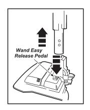
Caution: Do not attach or remove handle or wands while cleaner is ON. This could cause sparking and damage the electrical contacts.
